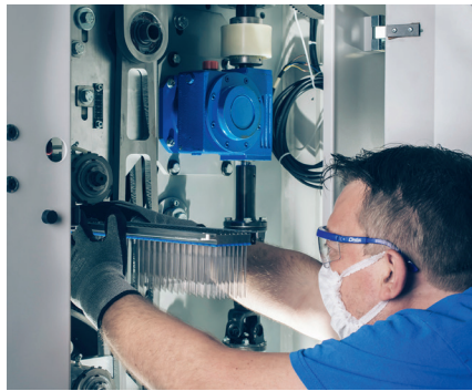
Easy access for operators and pneumatic clamping system
